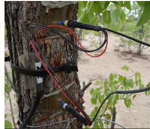
Installation of data logger and sensors to measure water use of trees.
