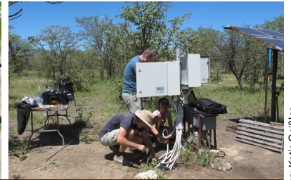
Installation of data logger and sensors to measure water use of trees.
